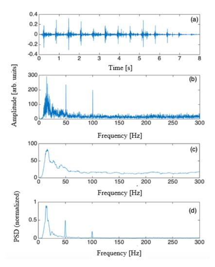
Figure 3. The horse footsteps (a) in time domain (b) in frequency domain (c) as filtered and (d) PSD frequency domain.
