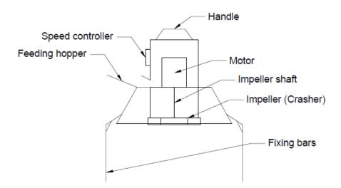
Figure 1. Representation of Hazelnut Cracking Machine
