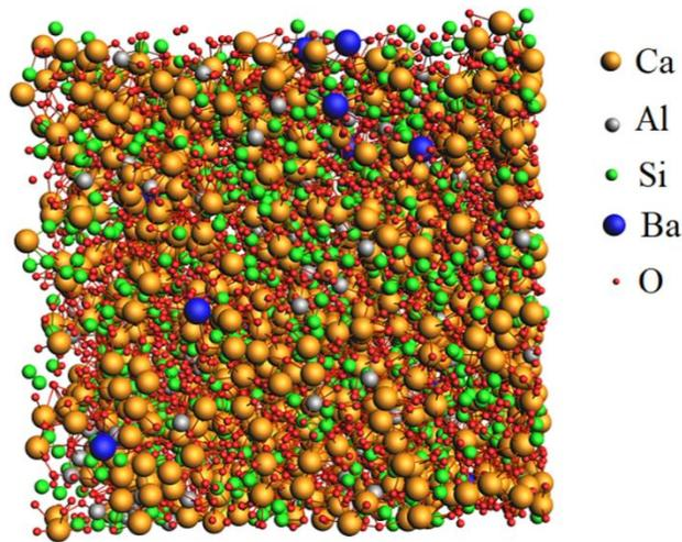
**Figure 3.** The simulation result of  $\text{SiO}_2\text{-Al}_2\text{O}_3\text{-CaO-BaO}$  glass ceramic model system at 300 K (Al, Si, Ba, Ca, and O atoms are shown in grey, green, blue, yellow and red, respectively).
