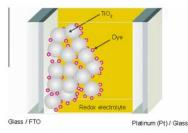
Figure 2. Typical structure of dye sensitized solar cell (Ahmad, 2015)
