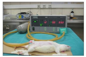
Picture 1. CO<sub>2</sub> was insufflated so as it remained in 6 mmHg
