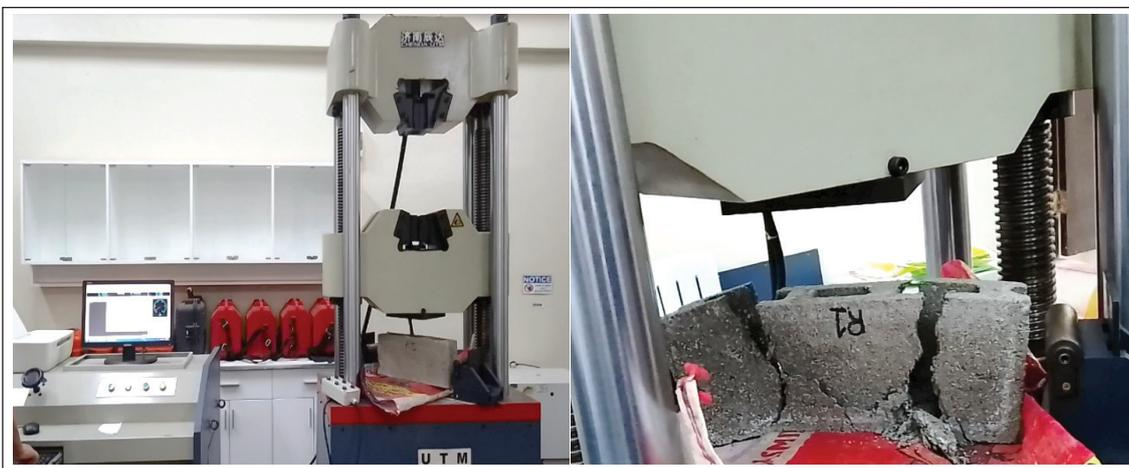
**Figure 3.** Compressive Testing of the Hollow Concrete Blocks through the UTM .
