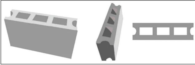
**Figure 2.** Hollow concrete block.
