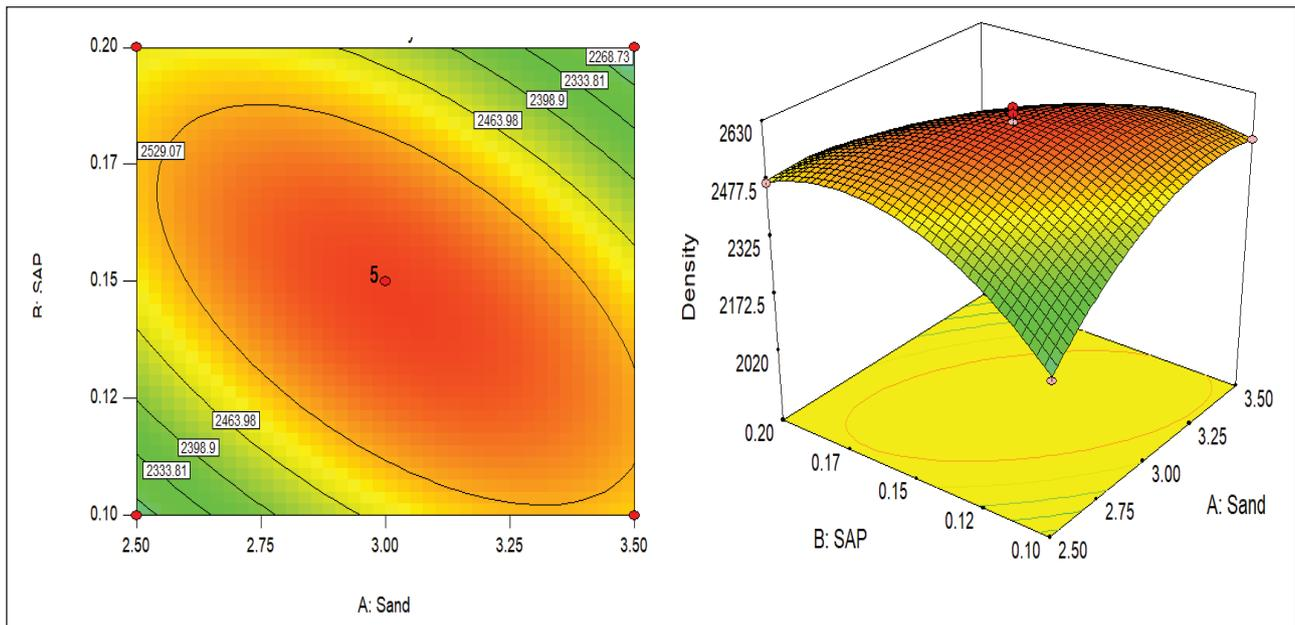
Figure 7. Contour and 3D Surface Plots of the Effects of Sand and SAP on Density.
