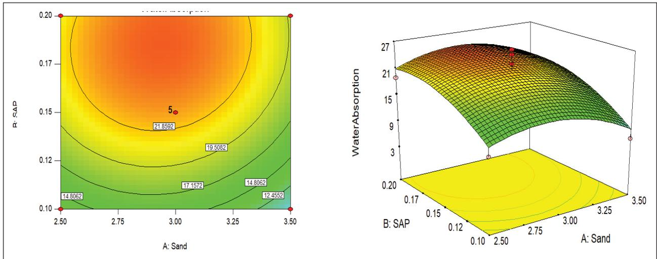
Figure 9. Contour and 3D Surface Plots of the Effects of Sand and SAP on Water Absorption.
