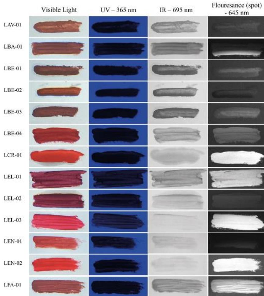
**Figure 1.** Liquid lipstick samples on VSC 8000 -1.
