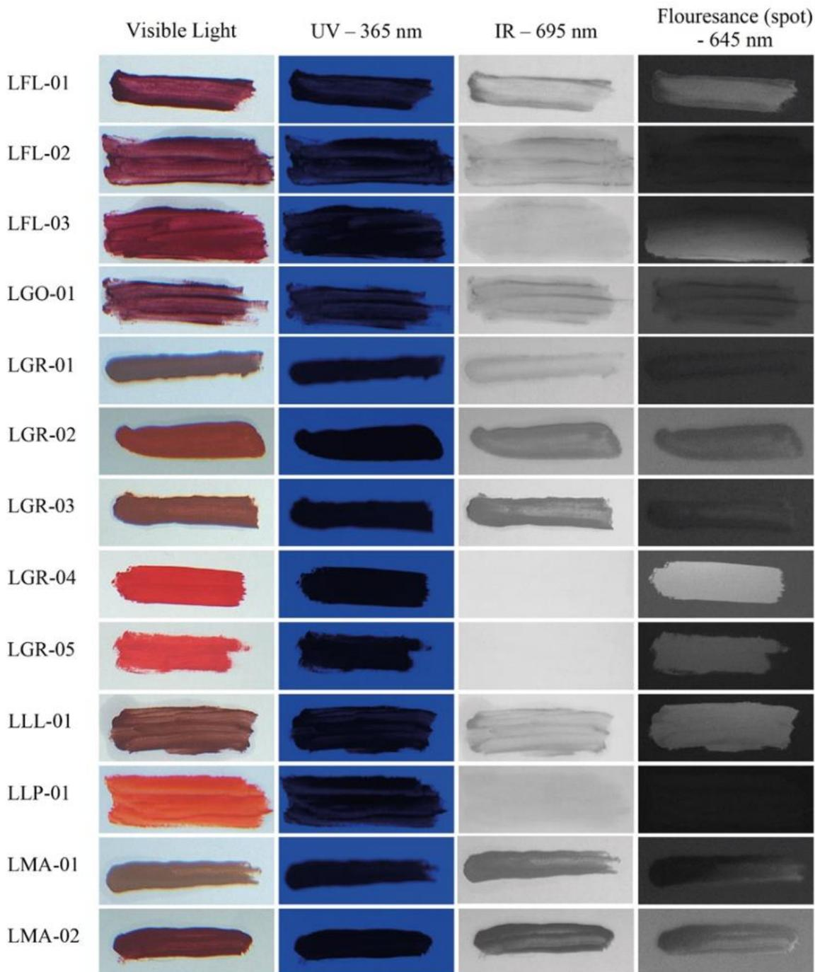
Figure 2. Liquid lipstick samples on VSC 8000 -2.
