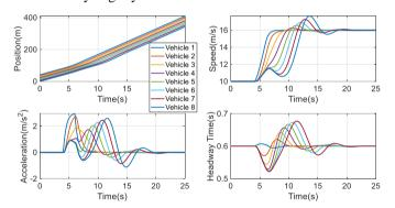
Fig. 7. CACC - Leader vehicle following simulation results
