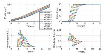
Fig. 8. CACC - Predecessor vehicle following simulation results
