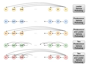
Fig. 4. Diagram of typical communication topologies [8]
