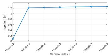
Fig. 13. Maximum intervehicle distance error for each vehicles in CACC-LF+PF convoy
