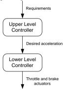
Fig. 1. General controller structure of ACC and CACC systems [9]
