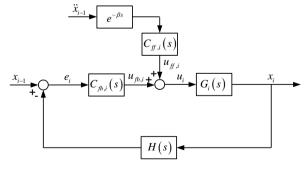
Fig. 3. CACC system structure for a single vehicle [1]
