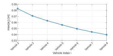
Fig. 12. Maximum intervehicle distance error for each vehicles in CACC-PF convoy
