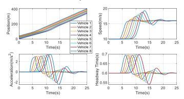
Fig. 6. ACC - Predecessor vehicle following simulation results
