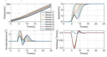
Fig. 9. CACC - Leader and predecessor vehicle following simulation results
