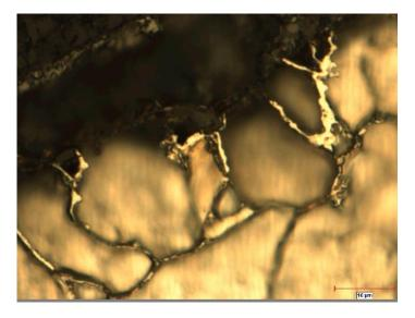
Figure 3. Industrial sample microstructural view of hot shortness.
