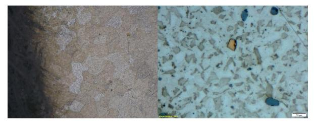
Figure 1. Microstructural view of Scientific 2 (Nital on the left, FeCl3 on the right).
