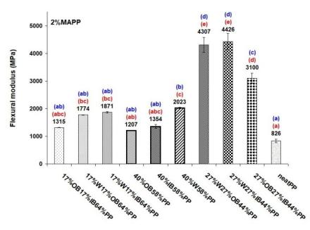
**Figure 2.** Mean values of flexural modulus of the IB/PP, OB/PP, W/PP, IB/OB/PP, IB/W/PP, OB/W/PP, IB/OB/W/PP and neat PP composites. Multiple range tests of Duncan that are indicated within parentheses demonstrate varying alphabetical designations highlighting significant differences among different treatments (composites). Red colour means at a 95% confidence level and blue colour means at a 99% confidence level.
