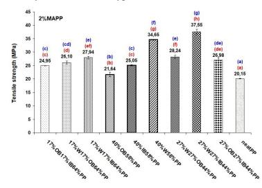
**Figure 3.** Mean values of tensile strength of the IB/PP, OB/PP, W/PP, IB/OB/PP, IB/W/PP, OB/W/PP, IB/OB/W/PP and neat PP composites. Multiple range tests of Duncan presented in parentheses signify distinct alphabetical designations that indicate significant disparities among various treatments (composites). Red colour means at a 95% confidence level and blue colour means at a 99% confidence level.
