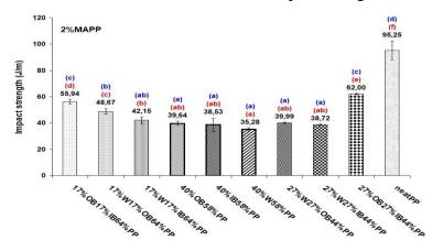
**Figure 5.** Mean values of impact strength of the IB/PP, OB/PP, W/PP, IB/OB/PP, IB/W/PP, OB/W/PP, IB/OB/W/PP and neat PP composites. Multiple range tests of Duncan indicated within parentheses denote distinct alphabetical designations underscoring significant disparities among various treatments (composites). Red colour means at a 95% confidence level and blue colour means at a 99% confidence level.
