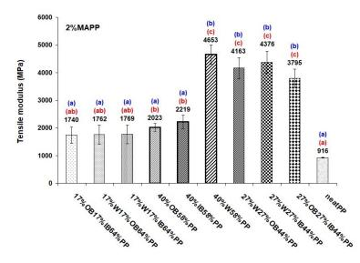
**Figure 4.** Mean values of tensile modulus of the IB/PP, OB/PP, W/PP, IB/OB/PP, IB/W/PP, OB/W/PP, IB/OB/W/PP and neat PP composites. Multiple range tests of Duncan presented in parentheses signify distinct alphabetical designations that indicates significant disparities among various treatments (composites). Red colour means at a 95% confidence level and blue colour means at a 99% confidence level.
