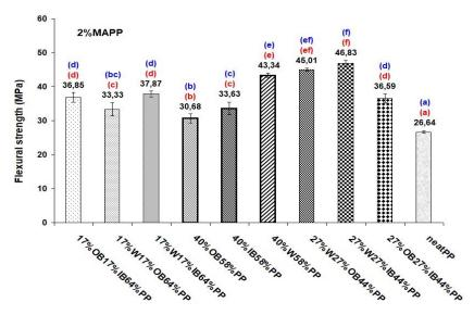
**Figure 1.** Mean values of flexural strength of the IB/PP, OB/PP, W/PP, IB/OB/PP, IB/W/PP, OB/W/PP, IB/OB/W/PP and neat PP composites. Multiple range tests of Duncan (in parentheses) reveal distinct alphabetical designations signifying significant differences among various treatments (composites). Red colour means at a 95% confidence level and blue colour means at a 99% confidence level.
