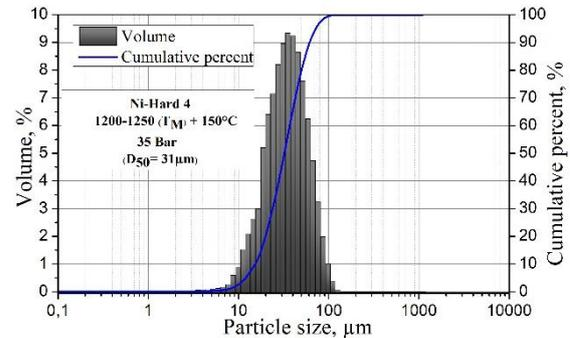
**Figure 4.** Particle size distribution graph of Ni-Hard 4 powders.
