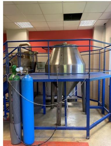
**Figure 1.** Gas atomization system used during experimental studies.
