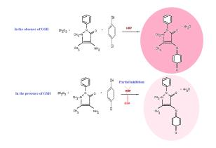
**Figure 1**. Working principle of the inhibition-based colorimetric glutathione determination method
