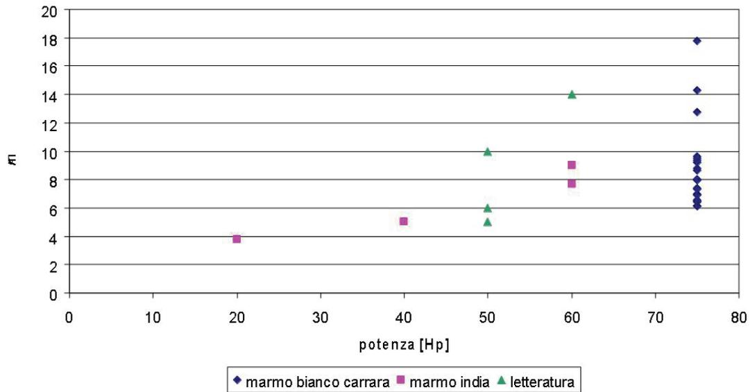
Figure 7 - Cutting rate against the power installed on the diamond wire saw.
