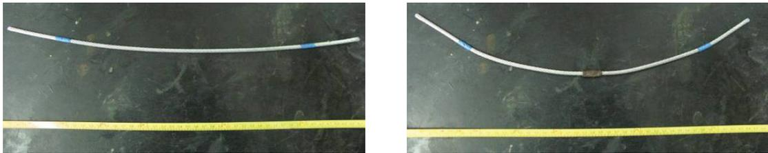
Figure 10 - Cable segments on which the test was performed (on the left, bare wire; on the right, cable with joint).
