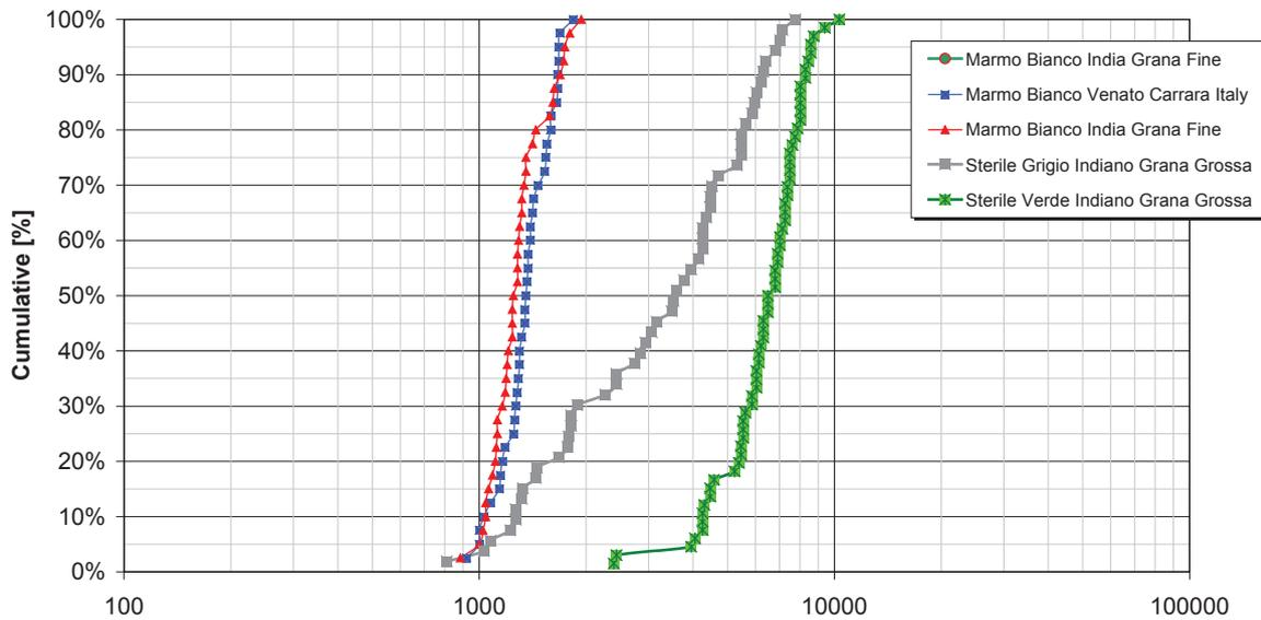
**Figure 4** - Microhardness frequency distribution diagrams of the rocks analyzed.
