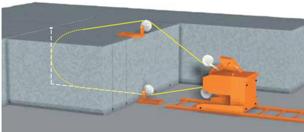
**Figure 5** - Scheme of a block cut in a quarry bench.
