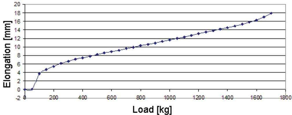
Figure 14 - Elongation of the cable as a function of load for the sample No. 2.
