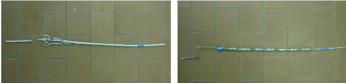
**Figure 11** - Samples of wire after fracture (bare wire on the left, the cable “covered” on the right).
