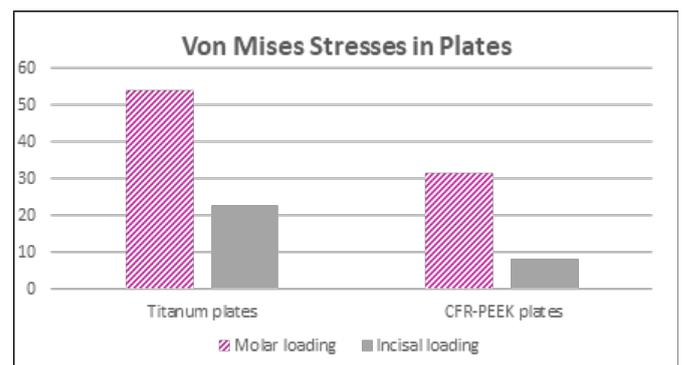
**Figure 2.** Von Mises stresses in plates
