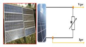
Fig. 6.UDTS50 Photovoltaic panels and assembly used to trace the external characteristic of the panels.
