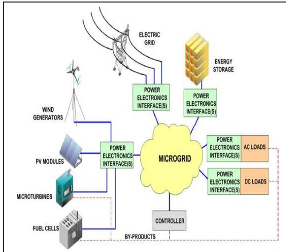
**Figure 1.** Structure of microgrid (Şimşek 2011).
