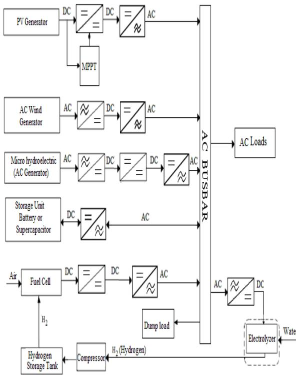
Figure 2. The block diagram of micro grid system
