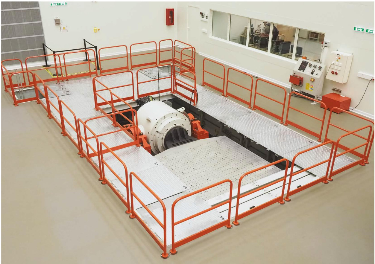
Figure 5. The vibration testing system with base isolation [1]
