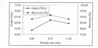
Figure 4b. Particle size on magnetic separation (at 575 °C)
