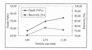
Figure 4a. Particle size on magnetic separation (at 550 °C)
