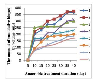
Figure 2. The change in cumulative biogas quantities
