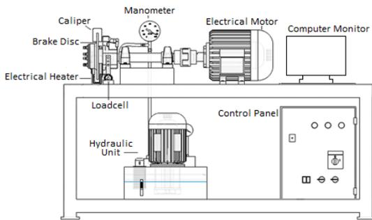
Fig. 2. Brake pad test device (Sugözü, 2015)
