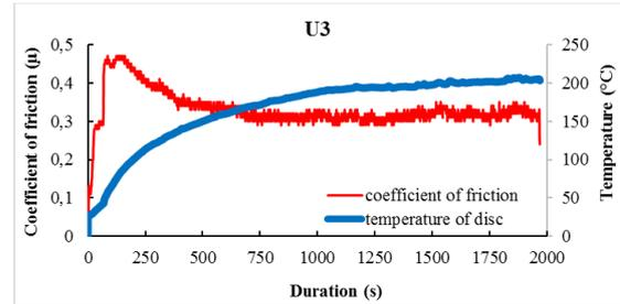
Fig. 3. The coefficient of friction and temperature graph of the specimen containing 3% ulexite, according to the friction time
