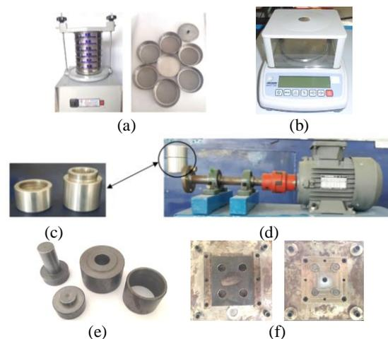
Fig. 1. The materials used in the production of specimens (a) the sieve-shaker and sieves (b) the precision scales (c) the powder chamber (d) the powder mixing device (e) the cold press mold (f) the hot press mold
