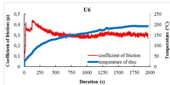
Fig. 4. The coefficient of friction and temperature graph of the specimen containing 6% ulexite, according to the friction time
