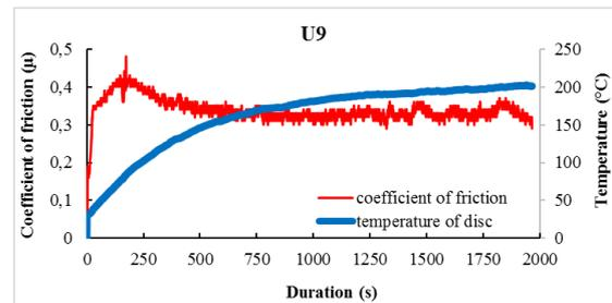
Fig. 5. The coefficient of friction and temperature graph of the specimen containing 9% ulexite, according to the friction time
