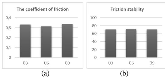
Fig. 6. (a) The coefficient of friction (b) friction stability graphs of specimens
