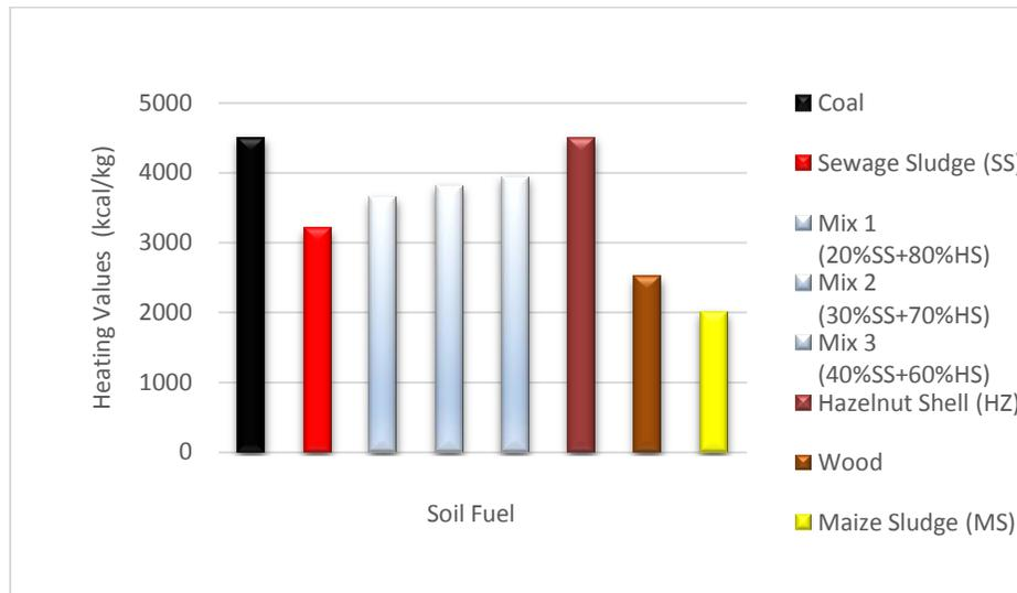
**Figure 4.** Heating Values of Solid Waste and Materials
