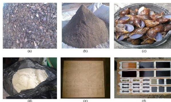
**Figure 1.** Photographs of the materials (a) as-received coconut shell (b) 150  $\mu\text{m}$  coconut shell particles (c) as-received snail shell (d) 150  $\mu\text{m}$  snail shell particles (e) wooden mould (f) some of the prepared composite samples in the mould.
