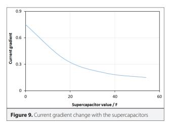
We formulated the supercapacitor induced change in current gradient as in equation 7, using curve fitting methods.
