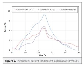
After these results, we investigated relation between the measured hydrogen consumption and expected hydrogen consumption from equations current value directly determines the hydrogen consumption.
