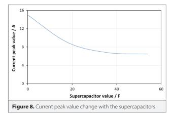
We formulated the supercapacitor induced change in peak current as in equation 6, using curve fitting methods.
