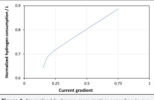
Figure 6. Normalized hydrogen consumption according to current gradient
