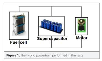
We performed same tests for supercapacitor values 18F, 36F and 54F. We measured the hydrogen consumption using Red-y flow meter.
