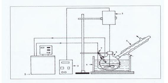
**Figure 1.** Experimental setup used in working processes. 1.Constant temperature circulator.2.Tachometer (Speed Adjuster), 3. Mechanical mixer, 4.Constant temperature bath, 5. Reactor, 6. Back-cooler, 7. Thermometer.
