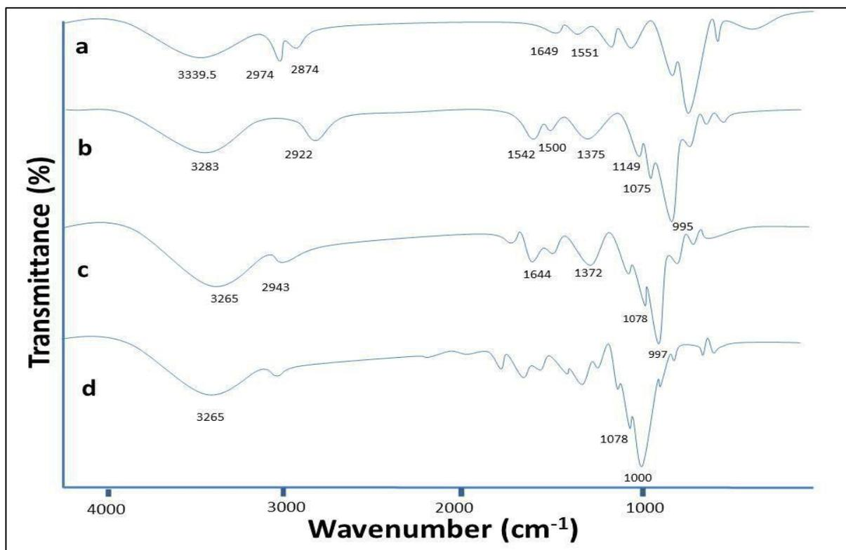
**Figure 3:** The FTIR spectrum of a. chitosan b. S1 (chitosan grafted starch) c. S2 (chitosan-graft-(starch; 2 g Pectin) films d. S3 (chitosan-graft-(starch; 5 g pectin) films.
