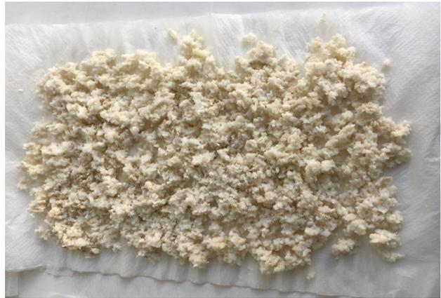
Figure 1. Paper pulp obtained with  $\text{NaClO}_2$  method
