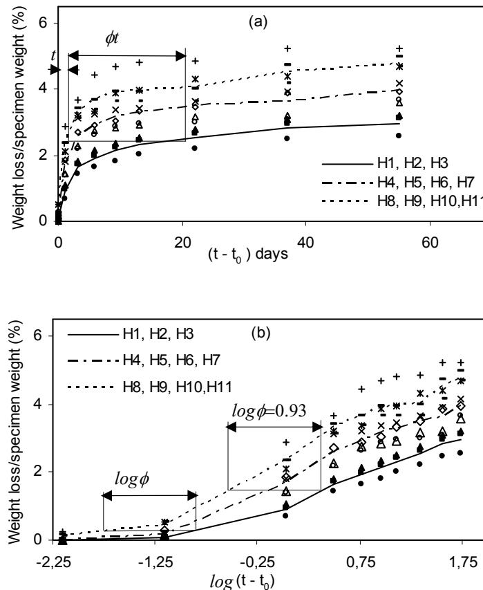
Figure 3. a) and b) Effect of size on weight loss with HSC.
