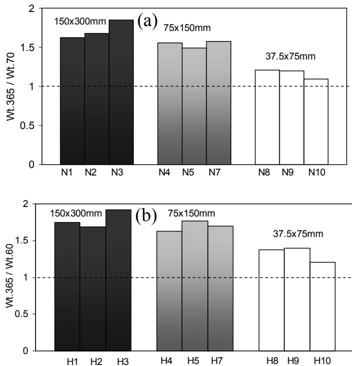
Figure 5. Comparison between long and short term results of weight loss a) for normal strength, b) for HSC.
