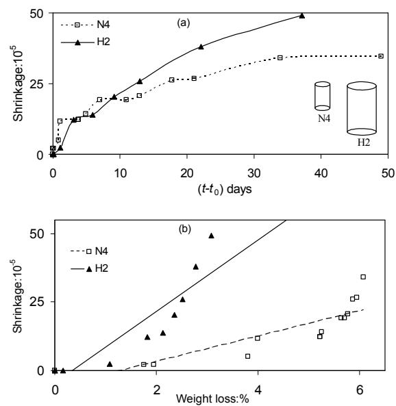
Figure 4. For HSC and normal strength cylinders, a) Effect of shrinkage, b) shrinkage-weight loss relationship.
