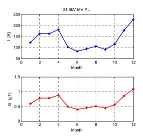
Fig. 7 Monthly based current load variation and magnetic flux for 31.5 kV MV-PDL.
