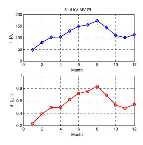
Fig. 6 Monthly based current load variation and magnetic field density for 31.5 kV MV-PDL.
