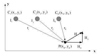
Fig.1. Magnetic field calculation for three conductor's lines
