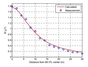
Fig. 8 Magnetic field variation form distance line center (at 1.5m height)
