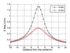
Fig. 3 EF variation depending on altitude for 34.5 kV MV-DPL.
