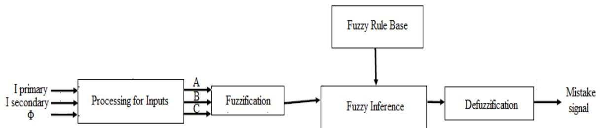
**Figure 2.** Fuzzy system for circuit breakers control.
