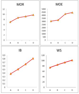
Figure 3. Properties of mechanical properties of the CBPBs.
