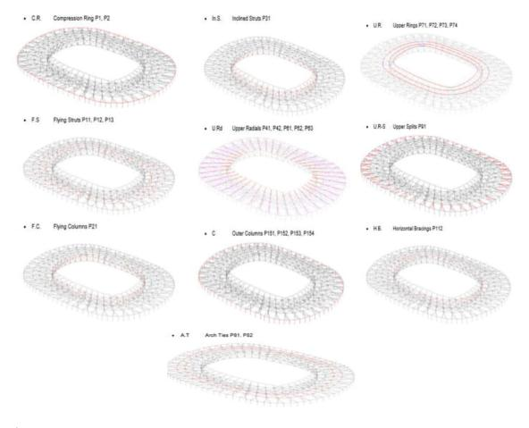
Figure 8. Steel frame elements.
