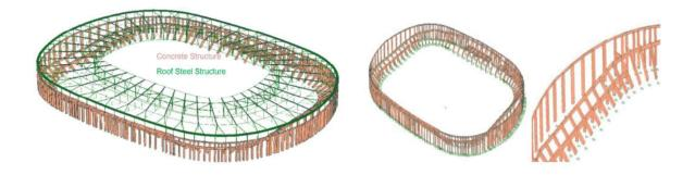
Figure 22. Concrete finite element model.
