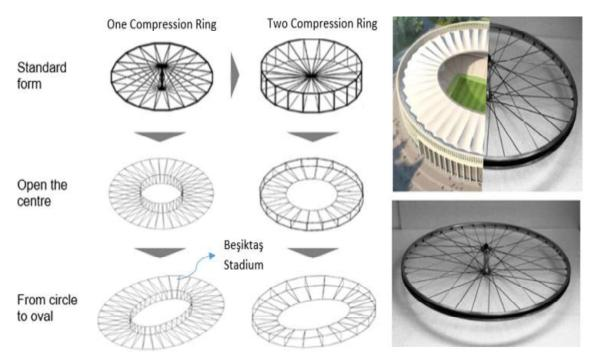
Figure 7. Typical bicycle wheel carrier system applications.
