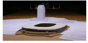
stadium roof of the proposed stadium against wind require the realistic assessment of the structular (areaaveraged) peak wind pressures acting on the roof, where both static and dynamic wind loads have to be considered.
