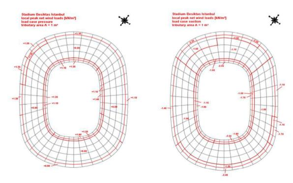
Figure 21. Local peak net wind loads for the design (suction and pressure).
