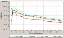
Figure 17. Solution residuals indictaing the error in different variables.
