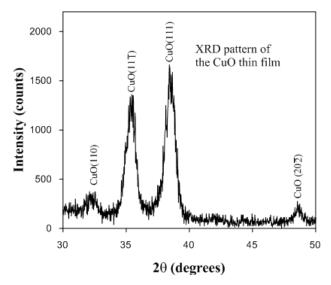
Figure 4. X-ray diffraction (XRD) measurements of CuO film produced at 250 °C substrate temperature.
