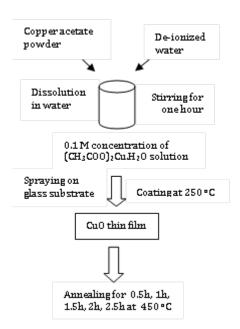
Figure 1.Schematic experimental diagram of spray coating system for CuO thin films.
