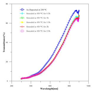
Figure 2. The optical transmission (T %) spectra of CuO thin film as deposited and annealed at 450 °C temperature.
