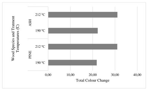
Figure 3. Total colour change caused by heat treatment process
