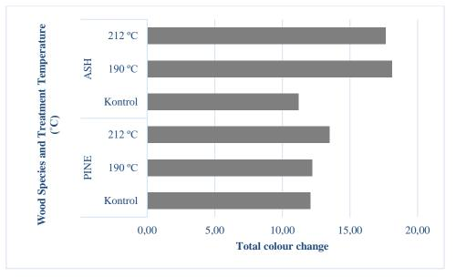
Figure 4. Total colour change caused by varnish apply
