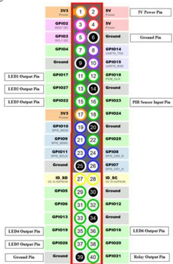
Figure 11. GPIO pins layout for proposed system
