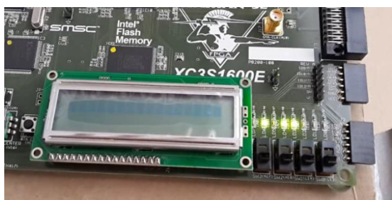
Figure 6 Display of 88 in binary at LED output of the FPGA
