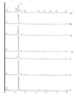
Figure 7. Fired wall tiles sample's XRD patterns (Q: Quartz. M: Mullite. P: Plagioaclase. )
