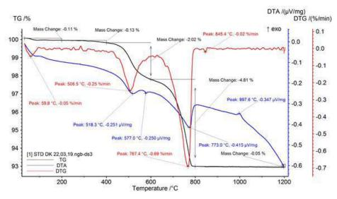
Figure 9. Thermogravimetric analysis of standart receipe
