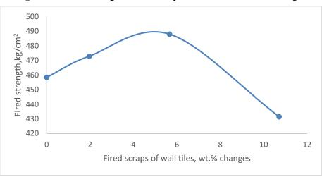
Figure 3. Fired strength- fired scraps of wall tiles wt. % changes
