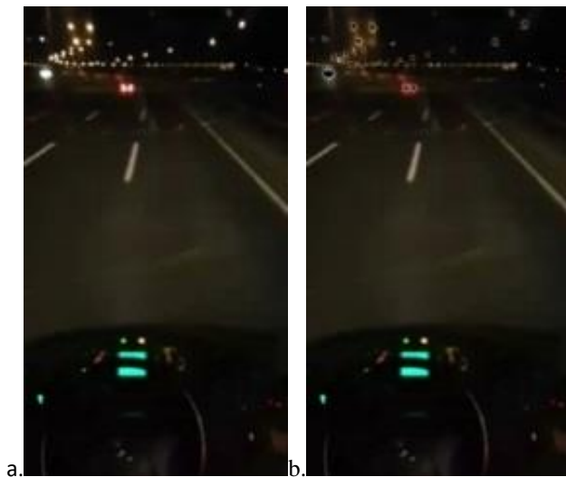
Fig.1. night road image a - original image b - light sources filtered image [31]
