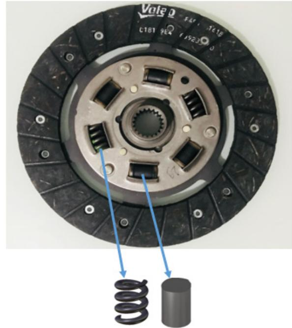
Figure 5. The prototype of hybrid damper clutch disc
