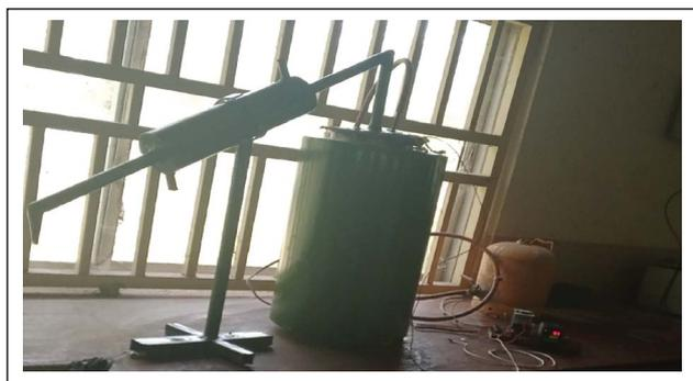
Figure 2. Co-pyrolysis system.
