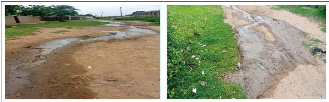
Figure 5. Water loss during pumping due to broken pipes within the city.
