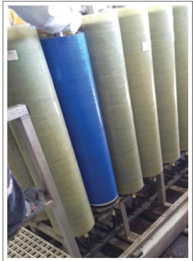
**Figure 9.** Unit 21 Disc membranes.
