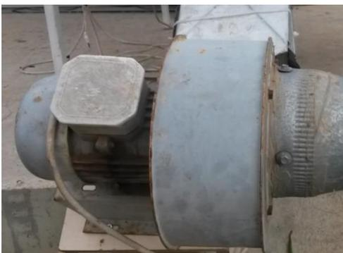
**Figure 10.** Motor and fan of the SAH.
