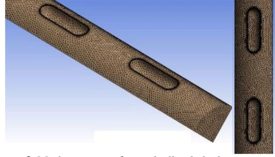
**Figure 3.** Mesh structure of capsule dimpled tube.
