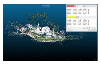
FIGURE 10. Rough alignment of LIDAR and photogrammetry point clouds.
