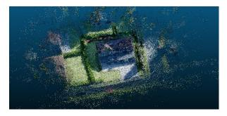
FIGURE 12. Concatenated point cloud using ICP algorithm.
