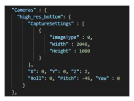
FIGURE 1. Drone camera parameters in AirSim.
