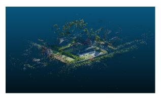
FIGURE 6. Colored point cloud formed by photogrammetry.
