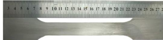
Figure 2. The tensile test specimen
