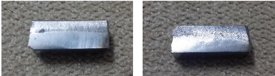
Figure 6. Charpy Impact Test Sample (after test)
