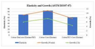
Figure 11. Elasticity (%) and growth (%) values in weft direction of denim fabrics (ASTM D3107-07)
