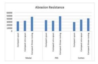
Figure 18. Abrasion resistance values of fabrics produced from compact spun, compact siro-spun and compact three-roving yarns
