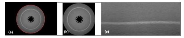
Figure 6. (a) Plotted bobbin boundary, (b) Image cropped according to bobbin outer boundary, (c) Bobbin cross-section extracted and transformed into rectangular image frame
