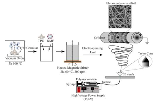
Figure 1. A detailed schematic illustration of the fabrication process of electrospun TPU and corresponding electrospinning unit
