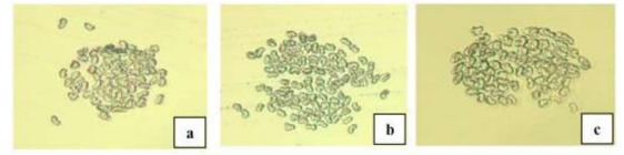
Figure 7. Cross section images of Modal yarns a) compact spun b) compact siro-spun c) compact three-roving
