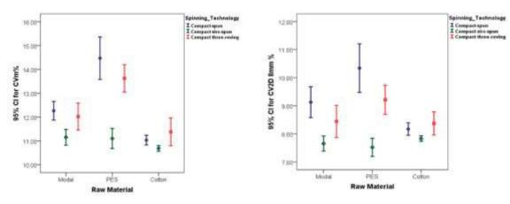
Figure 9. 95% confidence interval graphs for unevenness (CVm%) and optical unevenness (CV2D8mm%) values of compact spun, compact siro-spun and compact three-roving yarns
