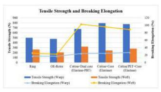
Figure 8. Tensile strength and breaking elongation of denim fabrics
