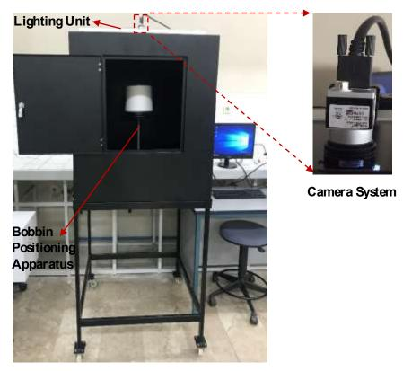
Figure 2. A prototype bobbin inspection cabin design
