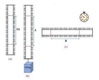
Figure 3. Calculation of fabric elasticity and growth (ASTM D3107-07)
