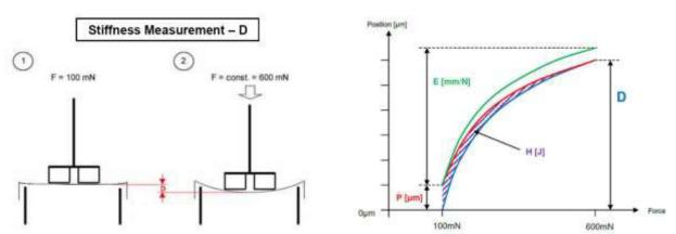
Figure 4. Measurement of the stiffness, elasticity, hysteresis and plasticity values [33]
