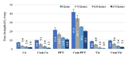
Figure 9. Tear strength of the fabrics (warp direction)
