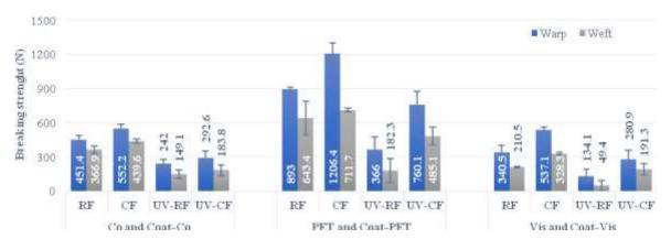
Figure 5. Breaking strength of raw and coated fabrics independent of UV exposure time for all fabric types
