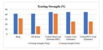
Figure 9. Tearing strength of denim fabrics
