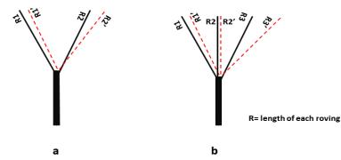
Figure 10. Geometrical changes of spinning triangles in siro-spun and three-roving yarns
