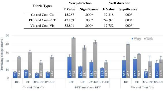
Figure 8. Breaking elongation of raw and coated fabrics independent of UV exposure time
