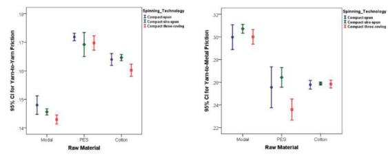
Figure 13. 95% confidence interval graphs for yarn-to-yarn and yarn-to-metal friction coefficients of compact spun, compact siro-spun and compact three-roving yarns
