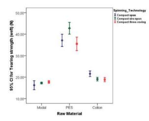
Figure 16. 95% confidence interval graphs for tear strength values of fabrics produced from compact spun, compact siro-spun and compact three-roving yarns
