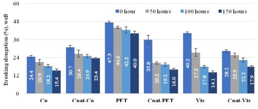
Figure 7. Breaking elongation of the fabrics (weft direction)
