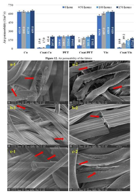
Figure 13. Deep cracks and ruptures observed on the raw cotton (a-1), coated cotton (a-2), raw viscose (b-1), coated viscose (b-2), raw PET (c-1), and coated PET (c-2) fabrics after 150 hours of UV exposure
