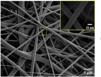
Figure 3. Morphology and structure of electrospun TPU fibers. Inset shows closer image of morphology of TPU fibers
