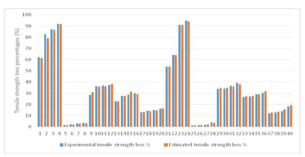
Figure 5. Comparison of results for estimated and experimentally observed tensile strength loss percentages of aramid fabrics
