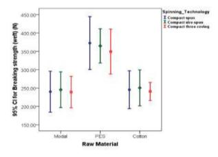
Figure 15. 95% confidence interval graphs for breaking strength values of fabrics produced from compact spun, compact siro-spun and compact three-roving yarns
