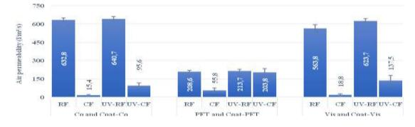
Figure 14. Air permeability of raw and coated fabrics independent of UV exposure time
