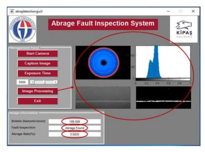
Figure 11. Abrage fault inspection system- User Interface
