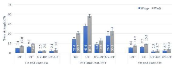
Figure 11. Tear strength of raw and coated fabrics independent of UV exposure time
