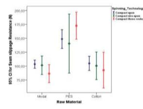
Figure 17. 95% confidence interval graphs for slippage resistance values of fabrics produced from compact spun, compact siro-spun and compact three-roving yarns
