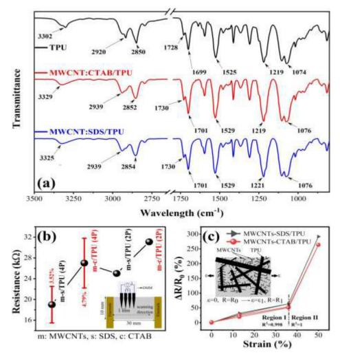
Figure 7. (a) FT-IR Spectra, (b) 2-point and 4-point probe resistance measurements and (c) uniaxial tensile strain measurement of electrospun MWCNTs-SDS/TPU and MWCNTs-CTAB/TPU samples. Inset figure in (b) and (c) shows the measurement setup for 4-point probe resistance measurement and piezoresistive working mechanism of electrospun sample under uniaxial tensile strain
