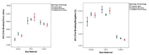
Figure 14. 95% confidence interval graphs for breaking force and breaking elongation values of compact spun, compact siro-spun and compact three-roving yarns
