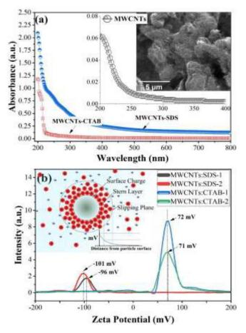
Figure 6. (a) UV-Vis spectra and (b) Zeta potential of MWCNTs-SDS and MWCNTs-CTAB dispersions. Inset figure in (a) shows UV- Vis and SEM image of non-dispersed MWCNTs and (b) shows the basic working principle of zeta potential
