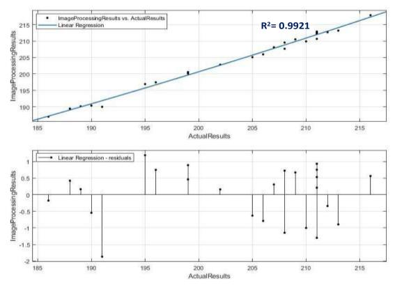
Figure 10. Q–Q plot of the actual and image processing measured bobbin diameter values (a) correlation graph, (b) residual graph of each measurement
