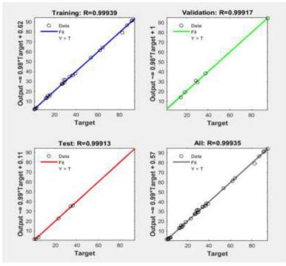
Figure 4. Results of the proposed MLP-ANN for tensile strength loss % (three hidden layers-5,5,5 neurons)
