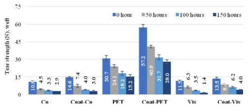
Figure 10. Tear strength of the fabrics (weft direction)
