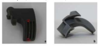
**Figure 4.** 3D printed suction-insert for compact three-roving yarn a) front view b) side view
