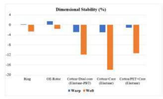
Figure 6. Dimensional stability of denim fabrics in warp and weft direction (%)
