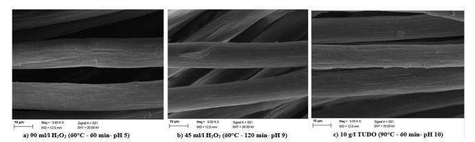
Figure 11. SEM images of bleached milk casein fabric samples. a) Peroxide bleaching under acidic conditions, b) Peroxide bleaching under alkaline conditions c) TUDO bleaching
