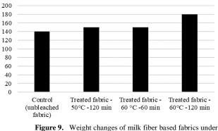
gure 9. Weight changes of milk fiber based fabrics under different processing conditions
