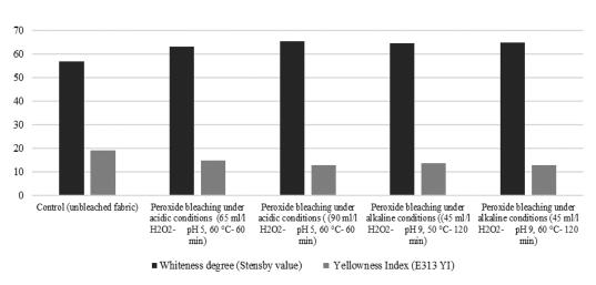
Figure 5. Peroxide bleaching of casein fabric under acidic and alkaline conditions
