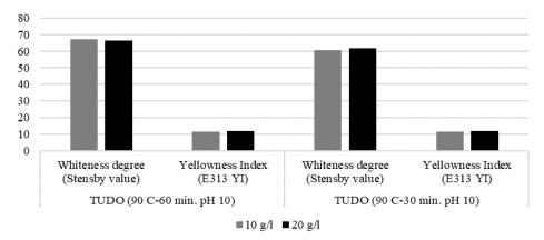
Figure 8. Effect of time on whiteness values of samples treated with TUDO at 90°C
