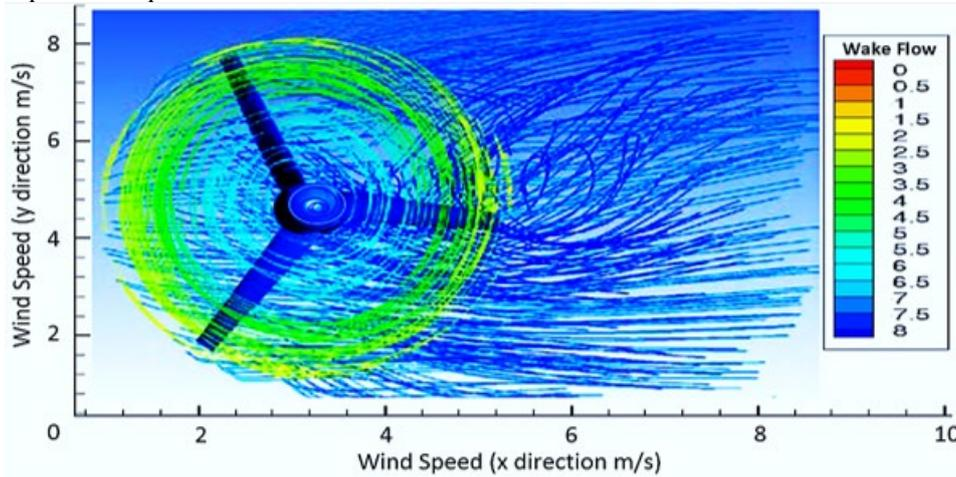
**Figure 5.** Wake distribution patterns behind the rotors
