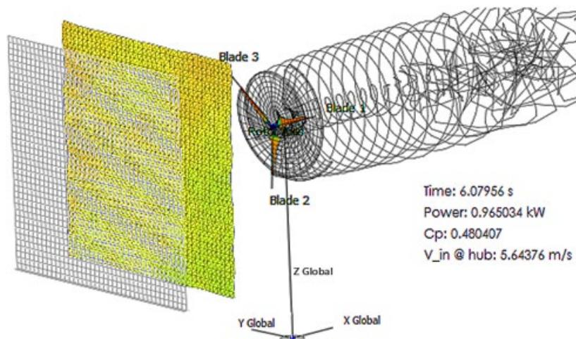
**Figure 9a.** Simulated profile of wake vortex trajectories at 6m/s
