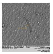
**Figure 10.** SEM image of LÇ<sub>11</sub> Electrospinning Fiber Formation.
