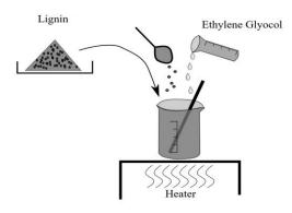
**Figure 4.** Schematic drawing figure of a preparing lignin-ethylene glycol blend.
