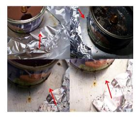
**Figure.8** The output of Lignin Fibers from the Perforated Chamber with Nozzle Function
