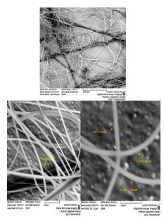
Figure 12. After electrospinning LB2 SEM Image.
