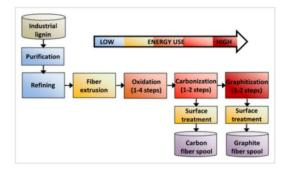
Figure 3. Lignin Carbon Fiber Extrusion [26].
