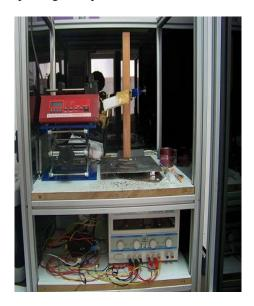
Figure. 9 Electrospinning Fiber Production Device.
