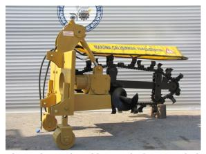
Figure 3 b. Trencher with a security frame attached
