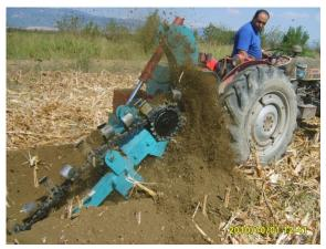
Figure 3 a. Engagement of the trencher in field (without security frame attached)
