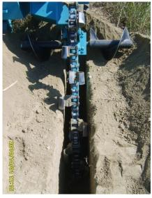
Figure 6. Spiral conveyors
