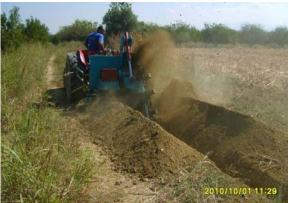
Technical specifications: The weight of trencher is 870 kg. Trencher has 4600 mm length, 92 links with 50 mm screw pitch endless-chain. Some technical specifications are given below:
