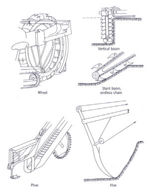
Figure 2. General classes of trenching machines (Frevert et al, 1955)
