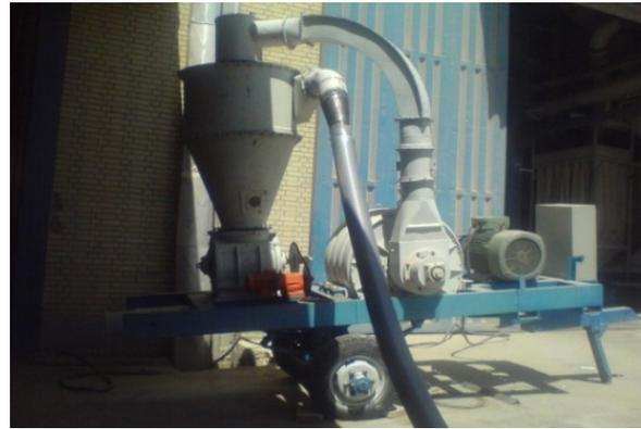
Figure 3. Pneumatic conveyer
