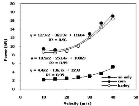
Figure 5. Effect of air velocity on the power consumption
