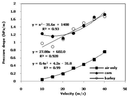
Figure 4. Effect of air velocity on the pressure drop
