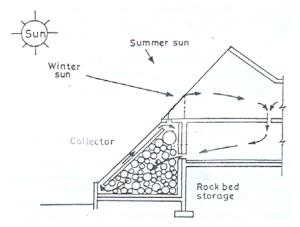
Fig. 2. The rock bed-passive solar system
