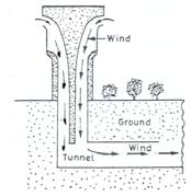
Fig. 3. The cross sectional view of an earth tunnel and wind tower
