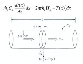
Fig. 4. Flow direction through an earth-air tunnel
