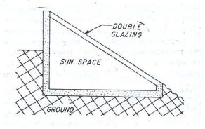
Fig. 1. The pit type structural design
