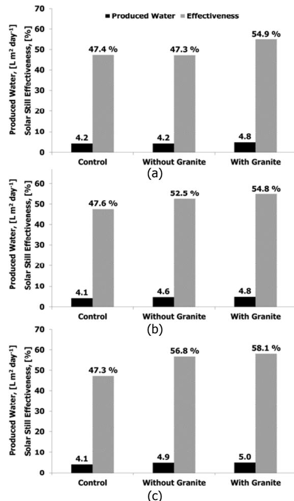
**Figure 2. Water production and solar still effectiveness of three solar stills; conventional (control), without and with granite solar absorbers under three treatments; (a) no cover cooling, (b) low flowrate and (c) high flowrate of cold water cooling.**
