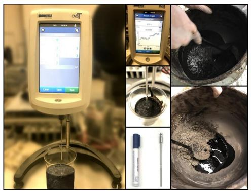
Figure 1. Sample preparation and viscosity test.
