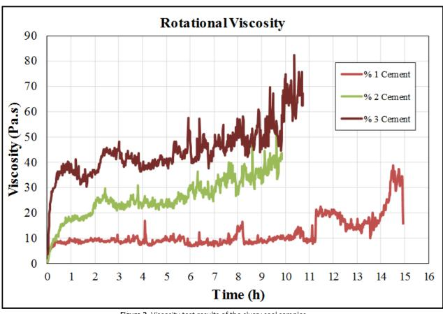
Figure 3. Viscosity test results of the slurry seal samples
